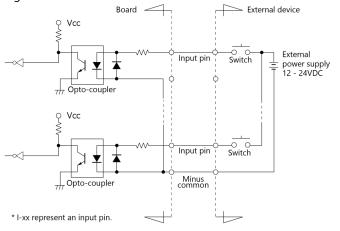
The input circuits of interface blocks of the DI-128RL-PCI is illustrated in the figure above.
