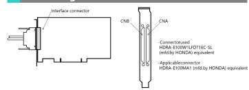
Layout on the Interface Connector(CNA, CNB)
