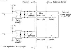
The signal inputs are isolated by opto-couplers (ready to accept current sinking output signals).
