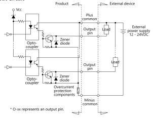
The signal output section is an opto-coupler isolated, open-collector output (current sink type). This product therefore requires the external power supply to drive the output section of this product.
