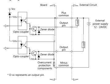
The signal output section is an opto-coupler isolated, open-collector output (current sink type).
