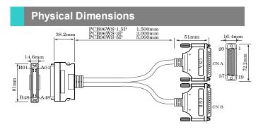
These products are cables which converts 96-pin half-pitch connector on CONTEC board into 37-pin D-SUB female connector.
