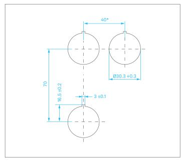
\* Recommended distance for mushroom pushbutton, emergency switch as well as position selector with protective shroud: 100 mm.
